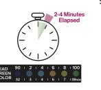
5. After **2-4 minutes** have elapsed, check the temperature strip label. A green color will appear to indicate the temperature of the urine specimen. The proper range for an unadulterated specimen is 90-100°F (32-38°C).
