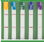
Two colored bands appear on the membrane. One band appears in the control region (C) and another band appears in the test region (T).
